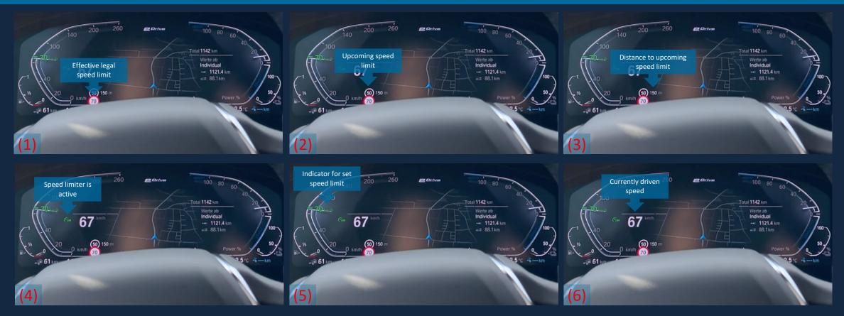
When the speed limiter is active, the acceleration pedal is not accepting foot pressure to accelerate the vehicle over the speed limit. Pressing the accelerator significantly will disable the limiter and accelerate the vehicle. An icon in the cluster is blinking as a visual warning.
