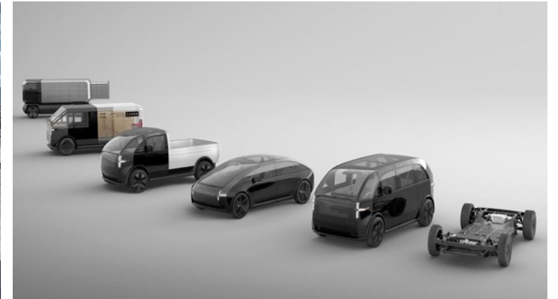
Electric vehicle startup Canoo's skateboard-style platform
